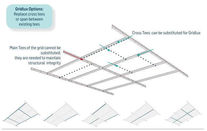
Gridlux replaces a standard cross tee or spans between tees. Therefore: To run Gridlux parallel to cross tees; replace cross tees with 1200mm Gridlux (Maintains a standard 1200x600 tile module) To run Gridlux parallel to the main tee; run a 600mm Gridlux between two cross tees to create a 600x600 module Various patterns can be created with a combination of the configurations outlined above.
